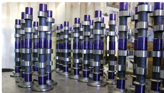
A non-metallic thermal coating is applied to every Eagle Camshaft.
