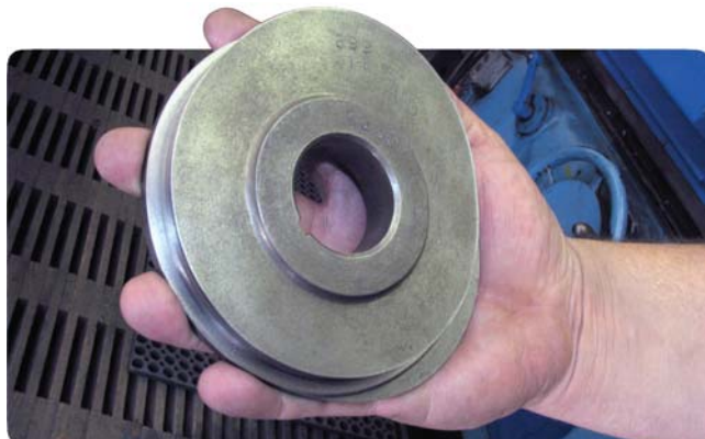
The Master Cam is a solid piece of tool steel.
